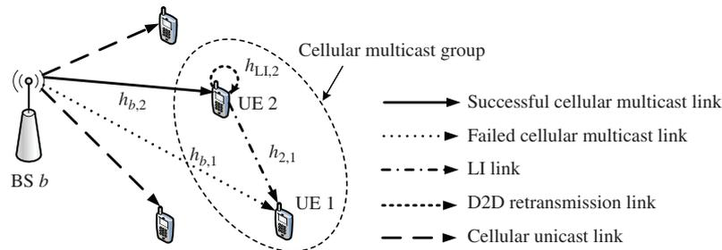
Figure 1 FD relaying based D2D retransmission model.
