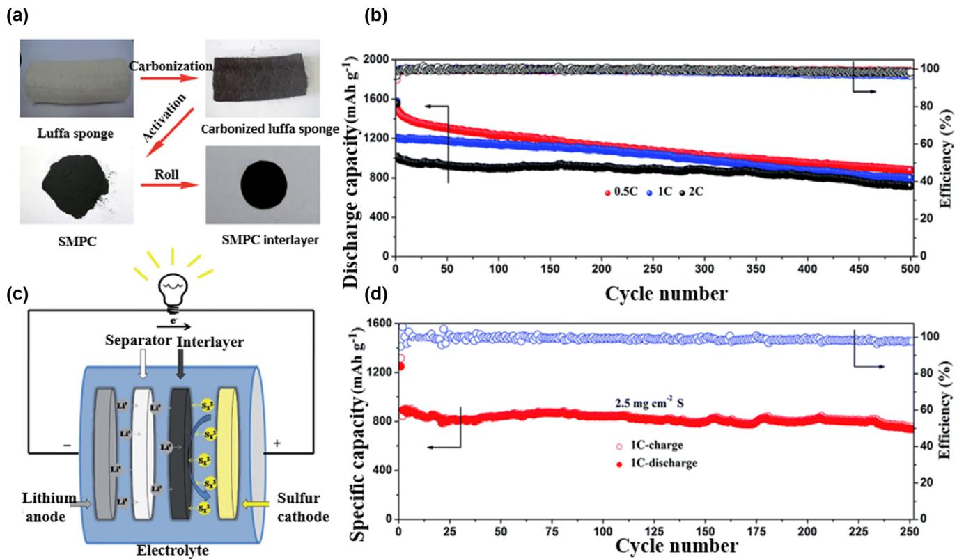
**Fig. 10.** (a) Schematic illustration for the formation of the SMPC interlayer. (b) Schematic cell configuration of the Li-S battery with SMPC interlayer. (c) The long cycling performance of the Li-S batteries with the SMPC interlayer at 0.5, 1 and 2 C. (d) Cycling performance of the Li-S batteries with the SMPC interlayer at 1 C [105].
