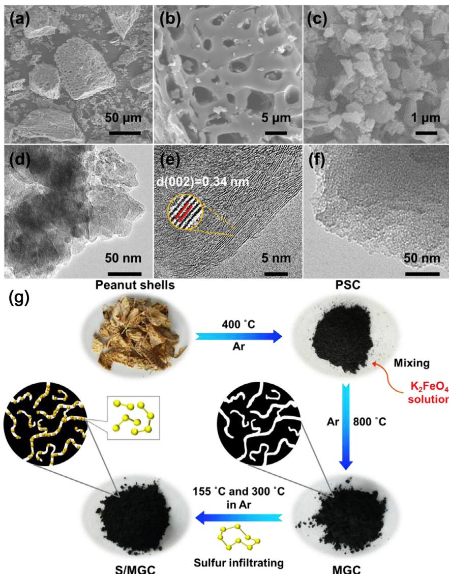
**Fig. 9.** SEM images of (a, b) MGC and (c) S/MGC; (d) TEM and (e) HR-TEM images of MGC; (f) TEM image of S/MGC; (g) the preparation process of the S/MGC composite [98].
