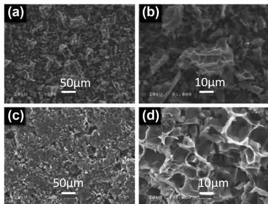
**Fig. 7.** SEM images of (a, b) the powder of cassava-carbon material (CCM) and (c, d) the surface of cassava-carbon sheets (CCS) [53].
