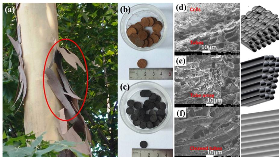
**Fig. 8.** Photographs of the fabrication process of integrated carbon slice electrodes: (a) bark of plane tree, (b) bark slices, and (c) carbonized bark slices; (d) FESEM image of outer layer and inter layer in carbonized plane tree bark and (e) its scheme. (f) Cross-section FESEM image of tube array and their schemes [101].
