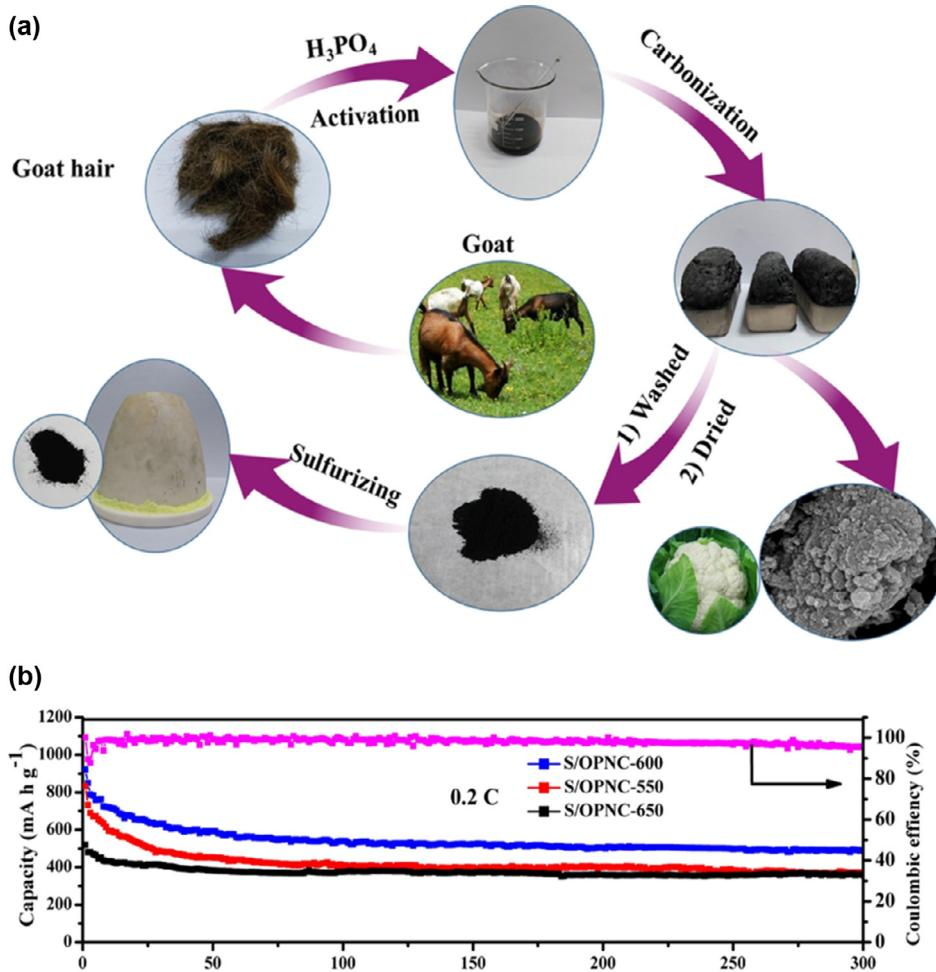
Fig. 12. (a) Schematic of the formation of S/NOPC composite materials; (b) Cycling performances of the S/NOPC-550, S/NOPC-600 and S/PPNC-650 composites at 0.2 C [84].
