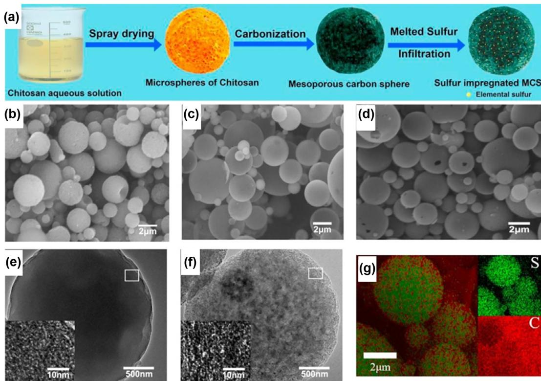
**Fig. 6.** (a) Illustration for the formation process of the S/MCS composite spheres; SEM images of MCS-0 (b), MCS-10 (c), MCS-20 (d) samples, TEM image of MCS-0 (e) and MCS-20 (f), and SEM image of S/MCS-20-50 (g) [97].
