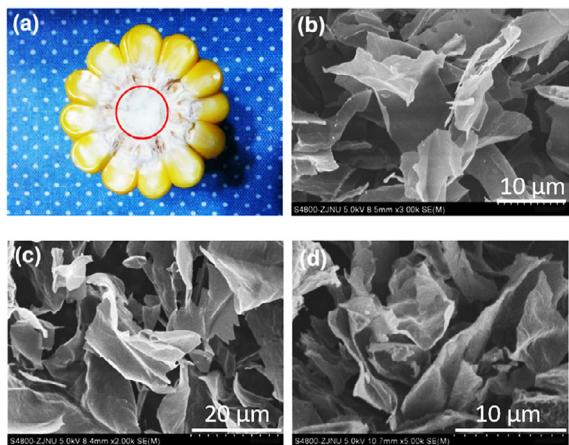
**Fig. 5.** (a) Digital photos of corn; (b, c, and d) SEM images of products carbonized at 500 and 900 °C from Ref. [55].
