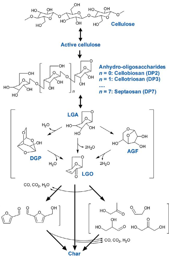
**Fig. 2.** Proposed mechanism of cellulose pyrolysis (DP indicates ‘degree of polymerization’) [65].
