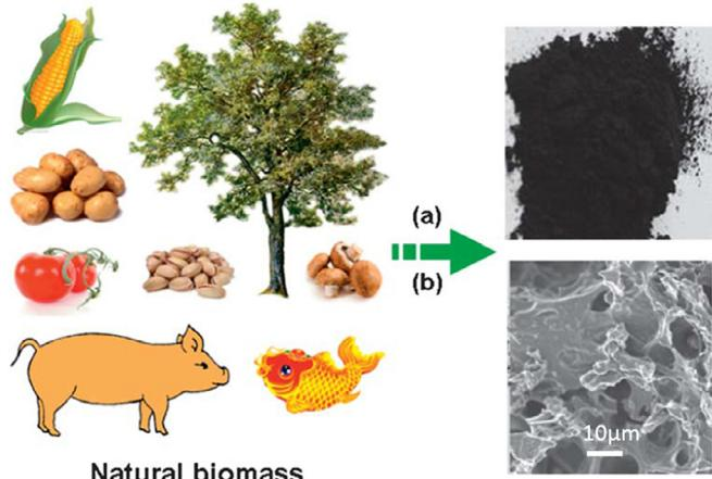
**Fig. 4.** Transformation of various natural biomass-derived materials into the ACs via (a) pre-treatment followed by (b) KOH activation [79].
