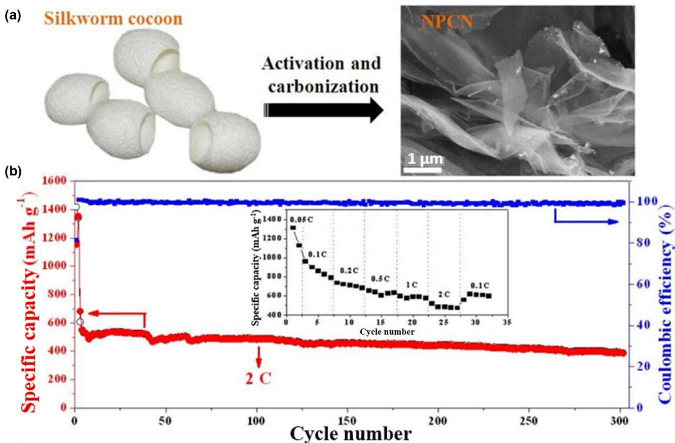
**Fig. 13.** (a) Schematic illustration of preparation processes of NPCN composites and (b) long-term cycling performance of the NPCN/S-55.7 electrode at a high rate of 2 C after two cycles at 0.05 C [51].
