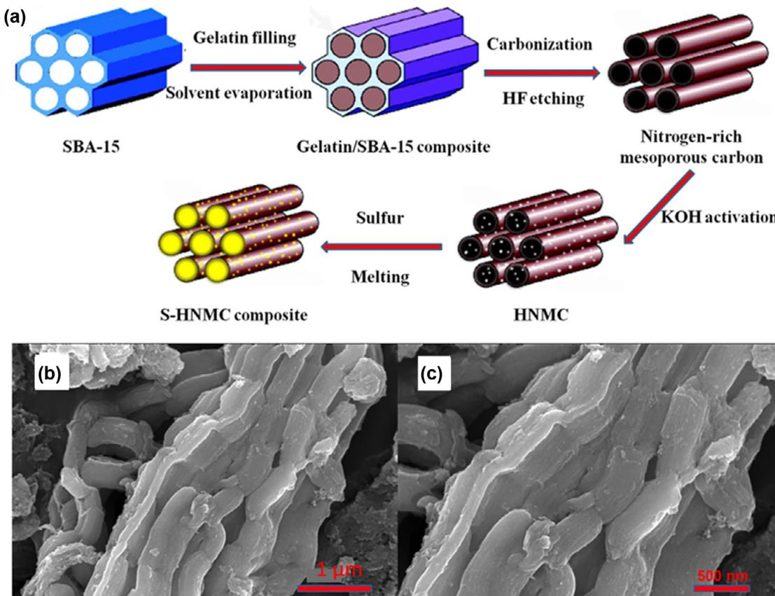
**Fig. 11.** (a) Schematic illustration of the synthesis procedure of the S-HNMC composite; (b, c) SEM images of the S-HNMC (53.3 wt% sulfur) composite [55].
