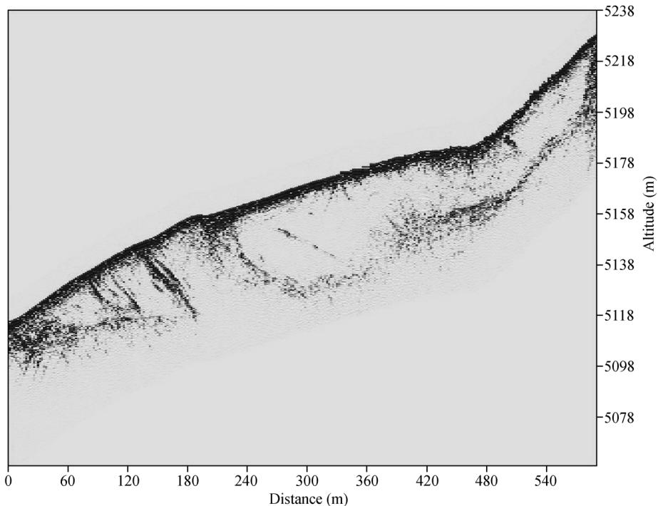
**Figure 4** The longitudinal profile of Glacier No.12 measured by 100 MHz GPR.
