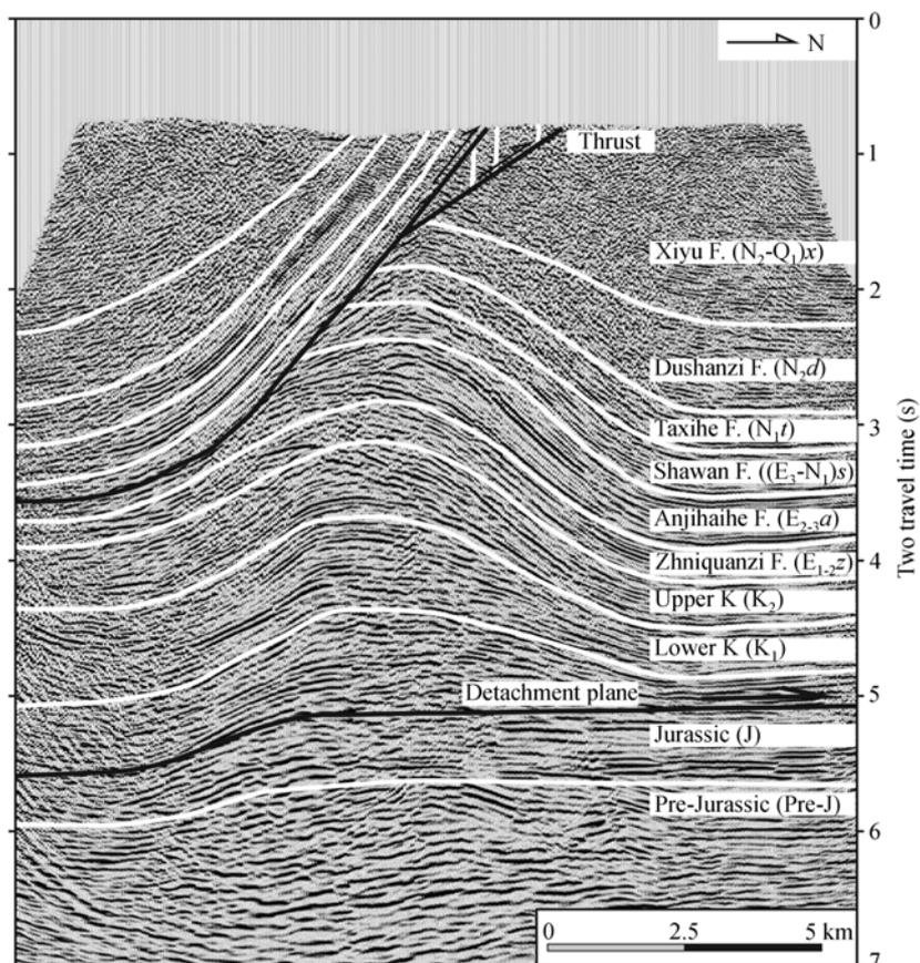
**Figure 3** The interpreted seismic profile crossing the Huoerguosi anticline, for locations see Figure 1.
