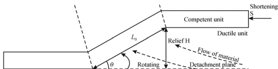
Figure 4 Geometrical model of progressive limb rotation<sup>[22]</sup>.
